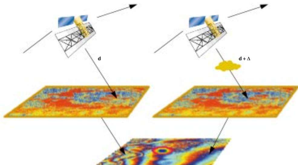
observe range changes at the centimeter level, the ionospheric effects must be removed almost completely.
