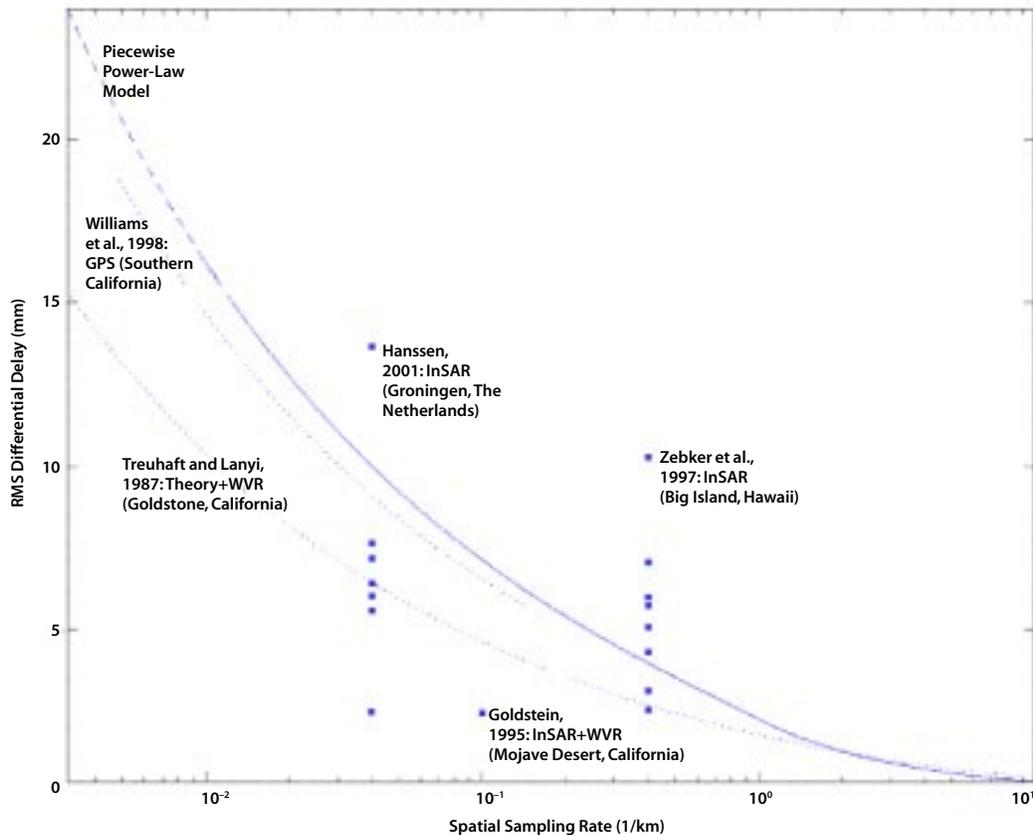
Figure 5.10 Residual one-way differential tropospheric zenith display comparing theoretical models and several data sets as calibration. The modeled residual wet tropospheric delay decreases with increased sampling rate.
